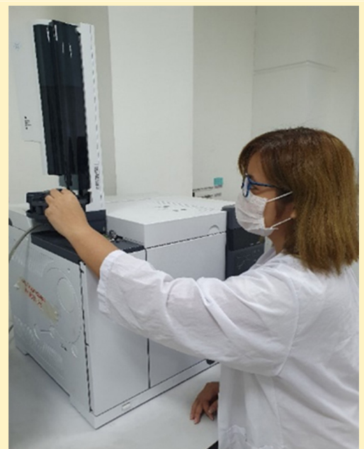
Analysis of nicotine and moisture component in smoke yield using Gas Chromatography
